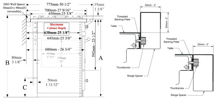
The 50mm range spacer is reversible using the alternate mounting holes on the opposite side of the spacer and the thumb screws provided, as shown above.
