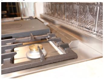
2. Flush-Mounted Position - [By UL Code Requirement] To use this spacer in the flush position: a heat & flame resistant backsplash material is mandatory (i.e. tile, stone or metal) - Simply mount the spacer to the rear lip of the rangetop using the provided mounting hardware as shown below. Then it follows the range as it is pushed up against a flat heat & flameproof backsplash surface (i.e. tile or stone).
